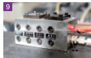
2 core pull standard, 2 reserved for easy later installation (268-568t)
